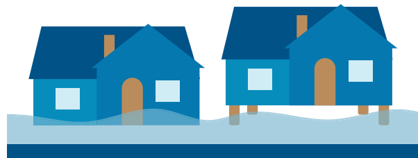
Figure 5. FEMA P-2022, MAT Report: Hurricane Harvey in Texas found that flood insurance claims of elevated homes required by current code were about 95% lower than non-elevated homes after Hurricane Harvey.
