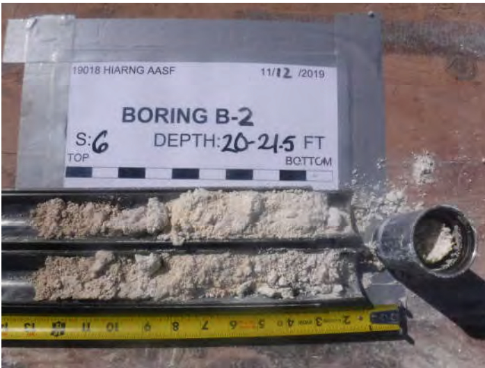
Boring B-2, Sample 6, Depth 20.0' - 21.5'
