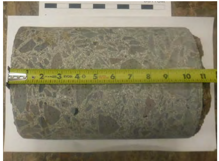
Boring B-2, Sample Core, Depth 0.0' - 1.0'
