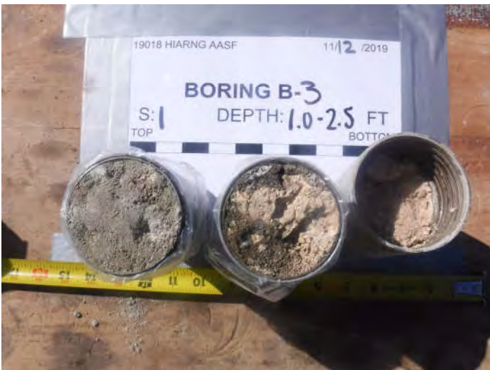
Boring B-3, Sample 1, Depth 1.0' - 2.5'
