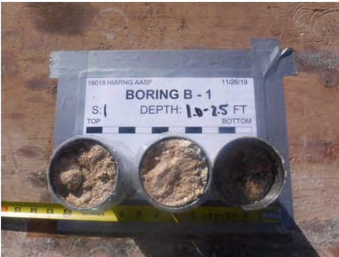
Boring B-1, Sample 1, Depth 1.0' - 2.5'
