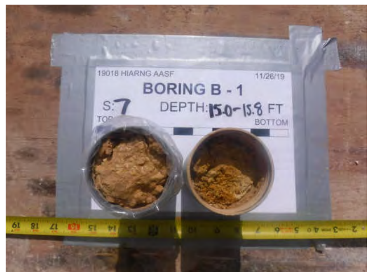
Boring B-1, Sample 7, Depth 15.0' - 15.8'
