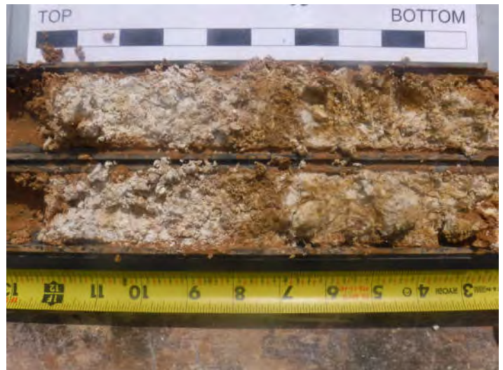
Boring B-1, Sample 8, Depth 15.8' - 17.3'
