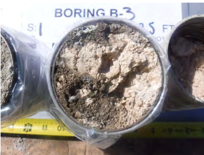
Boring B-3, Sample 1, Depth 1.0' - 2.5'
