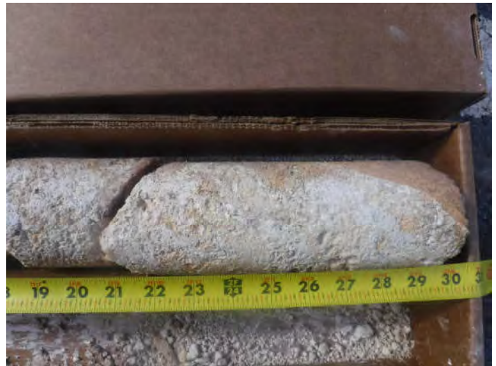
Boring B-1, Sample PQ-2, Depth 7.0' - 10.0'
