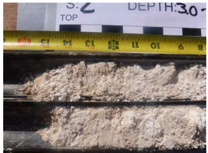
Boring B-1, Sample 2, Depth 3.0' - 4.5'
