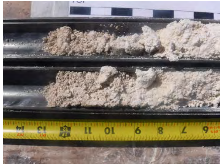
Boring B-2, Sample 6, Depth 20.0' - 21.5'
