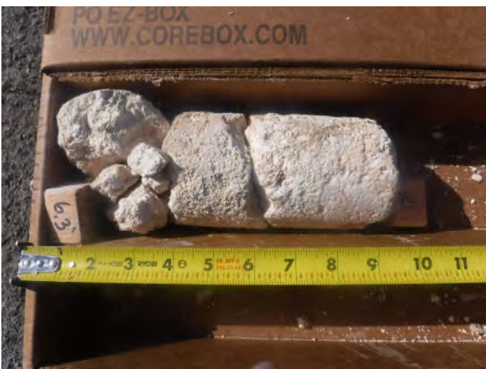
Boring B-1, Sample PQ-1, Depth 6.3' - 7.0'
