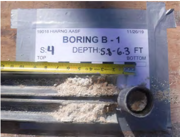
Boring B-1, Sample 4, Depth 5.8' - 6.3'
