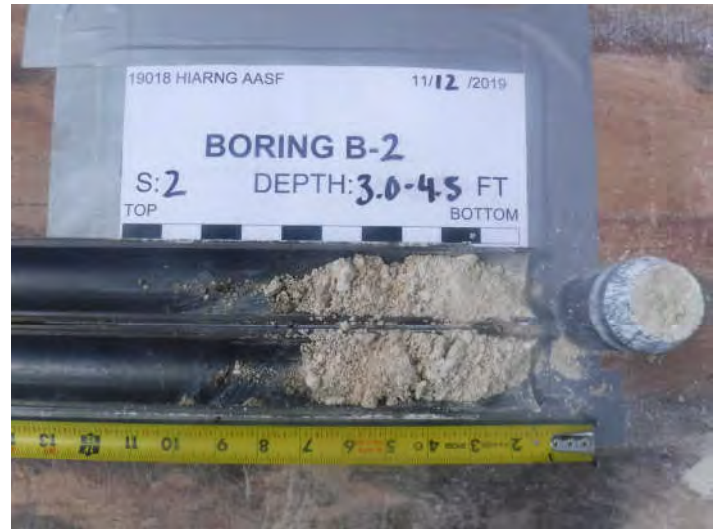
Boring B-2, Sample 2, Depth 3.0' - 4.5'
