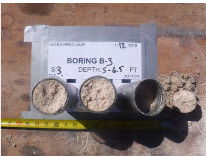
Boring B-3, Sample 3, Depth 5.0' - 6.5'
