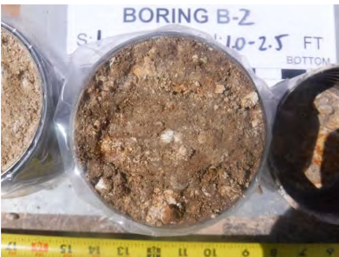
Boring B-2, Sample 1, Depth 1.0' - 2.5'
