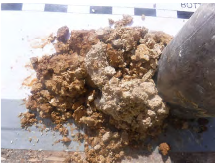
Boring B-1, Sample 5, Depth 10.0' - 10.3'
