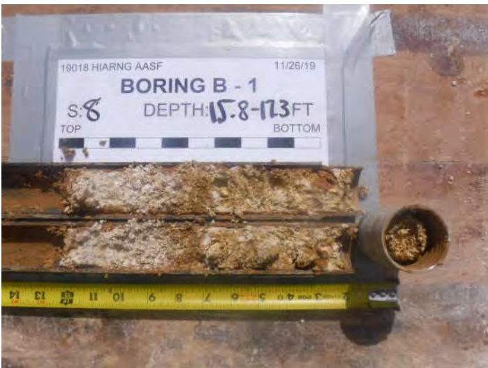
Boring B-1, Sample 8, Depth 15.8' - 17.3'
