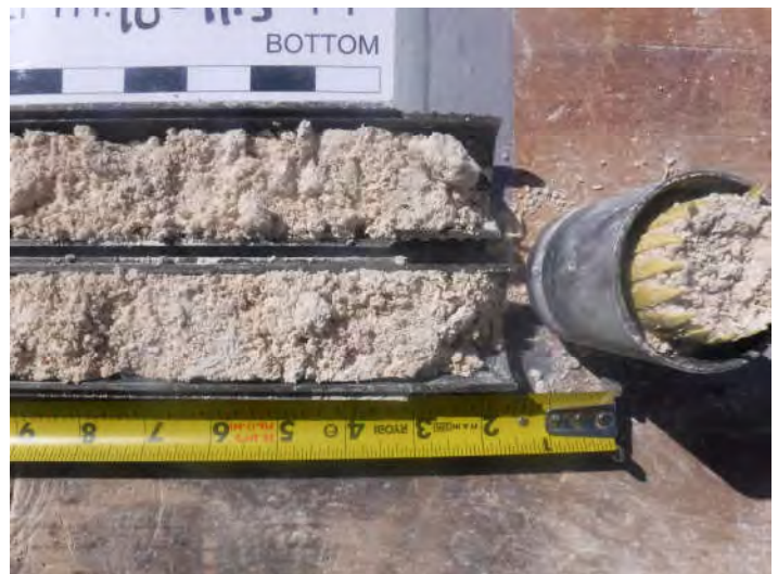
Boring B-3, Sample 4, Depth 10.0' - 11.5'
