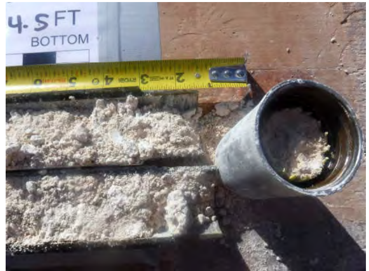
Boring B-1, Sample 2, Depth 3.0' - 4.5'
