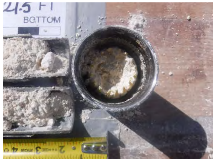
Boring B-2, Sample 6, Depth 20.0' - 21.5'
