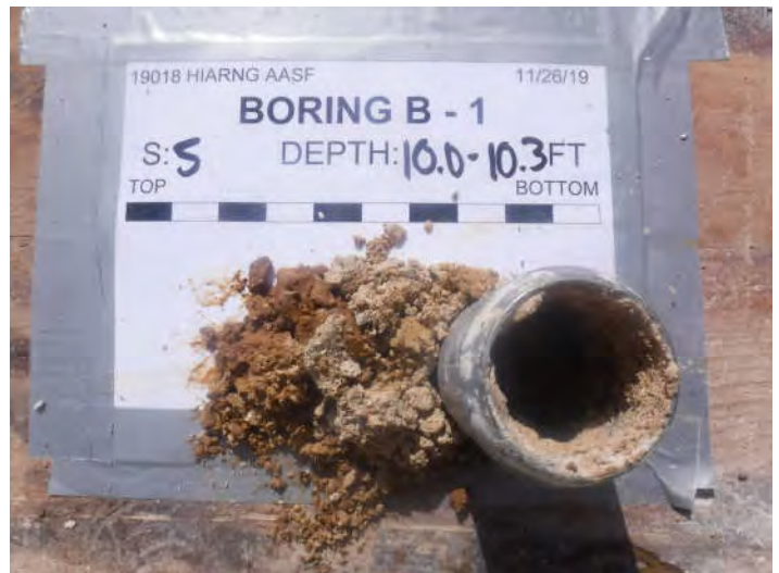
Boring B-1, Sample 5, Depth 10.0' - 10.3'
