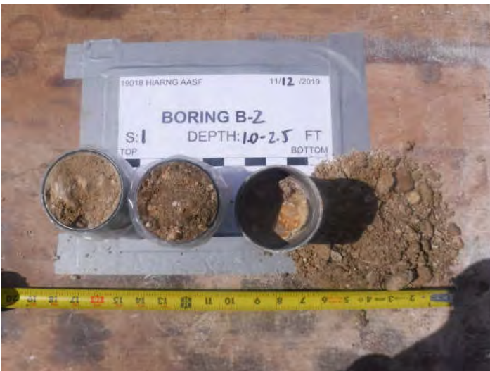
Boring B-2, Sample 1, Depth 1.0' - 2.5'
