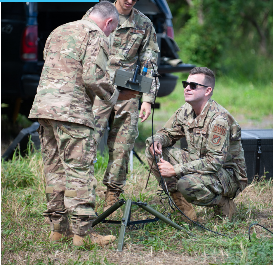
U.S. Air Force service members with the 199th Weather Flight, Hawai'i Air National Guard, set up a TMQ-53 Tactical Meteorological Observing System during aero-medical evacuation exercises with the 126th and 189th Aviation Regiments of the Hawai'i Army National Guard at Dillingham Airfield March 4, 2022. The TMQ-53 is a portable, automated weather station that can take observations in up to one-minute intervals, enabling flying missions from anywhere in the world. It collects weather data, that includes wind speed and direction, temperature, humidity, cloud height, precipitation and lightning. (U.S. Air Force photo by Senior Airman Robert Cabuco)
