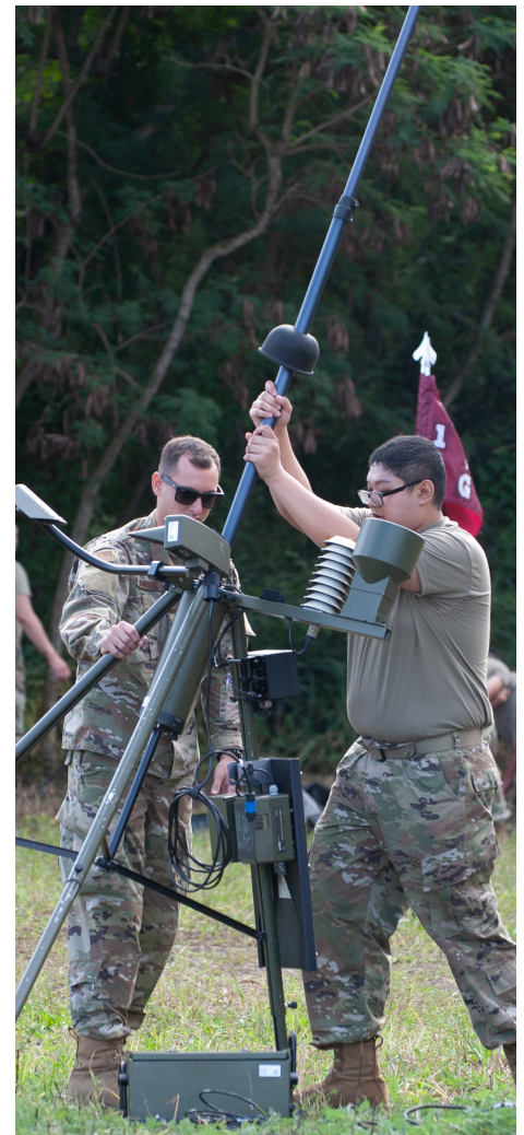
U.S. Air Force Senior Airman Adam Mattson and Senior Airman Alec Lagalog with the 199th Weather Flight, Hawai'i Air National Guard, set up a TMQ-53 Tactical Meteorological Observing System during aero-medical evacuation exercises at Dillingham Airfield March 4, 2022. The HIANG's 199th Weather Flight has a long-standing mission requirement to provide weather support to the 126th and 189th Aviation Regiments of the Hawai'i Army National Guard. (U.S. Air National Guard photo by Senior Airman Robert Cabuco)
