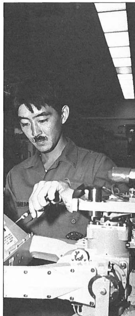
A 154th Consolidated Maintenance Squadron airman makes adjustments to the F-15's radar during ground testing.
