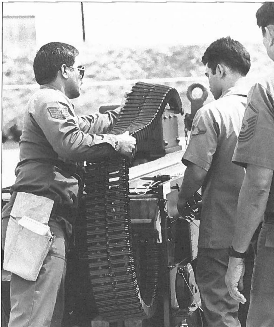
Munition technicians of the 154th Consolidated Maintenance Squadron load 20-mm rounds into ground servicing equipment prior to reloading an F-15 internal "Gatling" gun.
