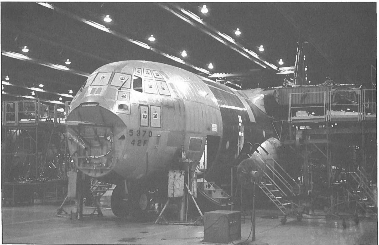
HERCULES UNCHAINED -- One of the Hawaii Air National Guard's new C-130H models awaits completion during its final leg of production at Lockheed Aeronautical Systems Company in Marietta, Ga.
