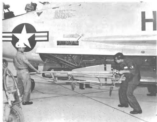
Rockets and guided missiles are loaded into belly of F-102 Delta Dagger at Hickam AFB.
