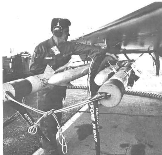
Staff Sgt. Gary Kodani insures that missiles are securely fastened to the F-4C on the alert pad.
