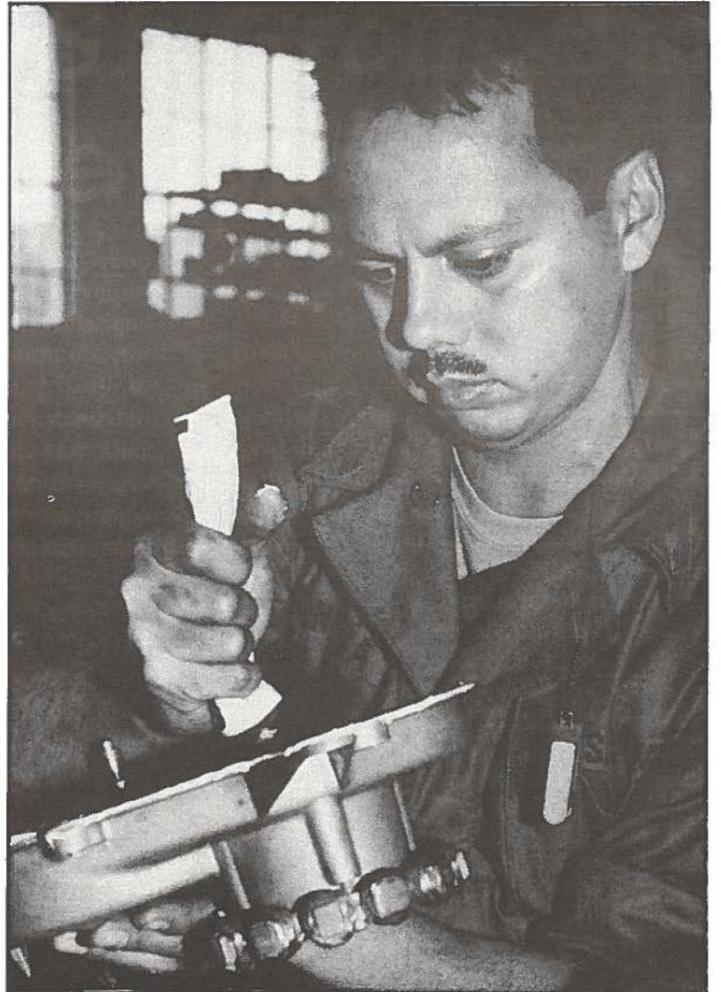
**Sgt. Anthony Villanueva**, of the 291st Maintenance Company, applies liquid gasket to a timing gear plate while rebuilding a generator at the Army's Equipment Maintenance Center-Europe in Kaiserslautern, Germany. The 291st rebuilt six generators at the facility during annual training, June 5-26.
