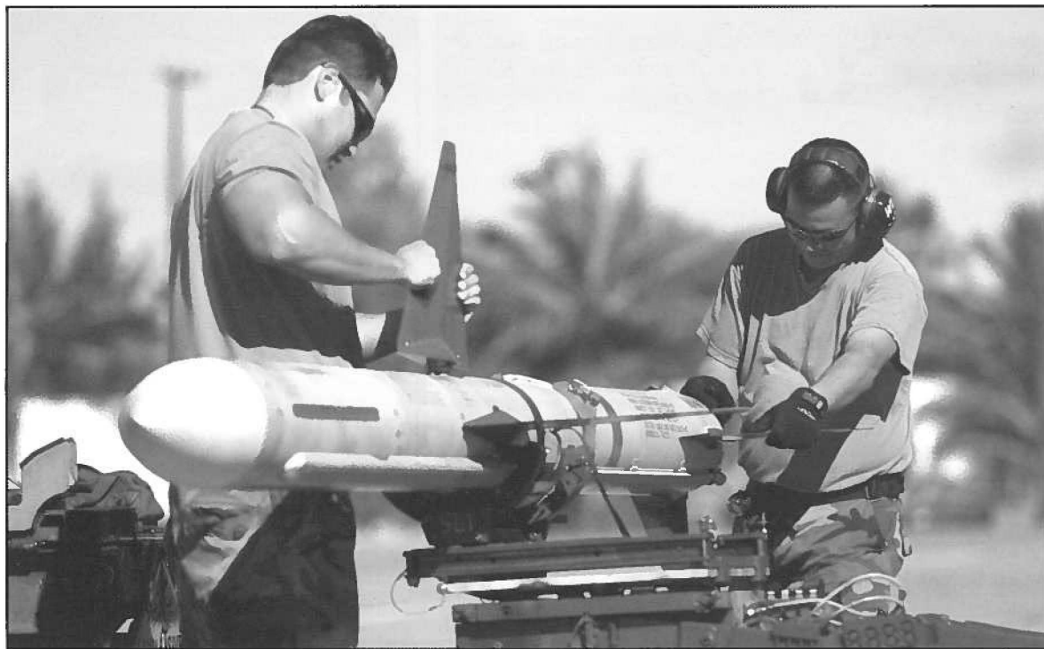
Staff Sgt. Gabriel Coronado and Staff Sgt. Arthur Hamabata install the wings and fins on an AIM-7 Sparrow missile at Hickam Air Force Base, Hawaii, on July 16 during the Rim of the Pacific Exercise 2006. The Airmen are from the Hawaii Air National Guard's 154th Aircraft Maintenance Squadron.
