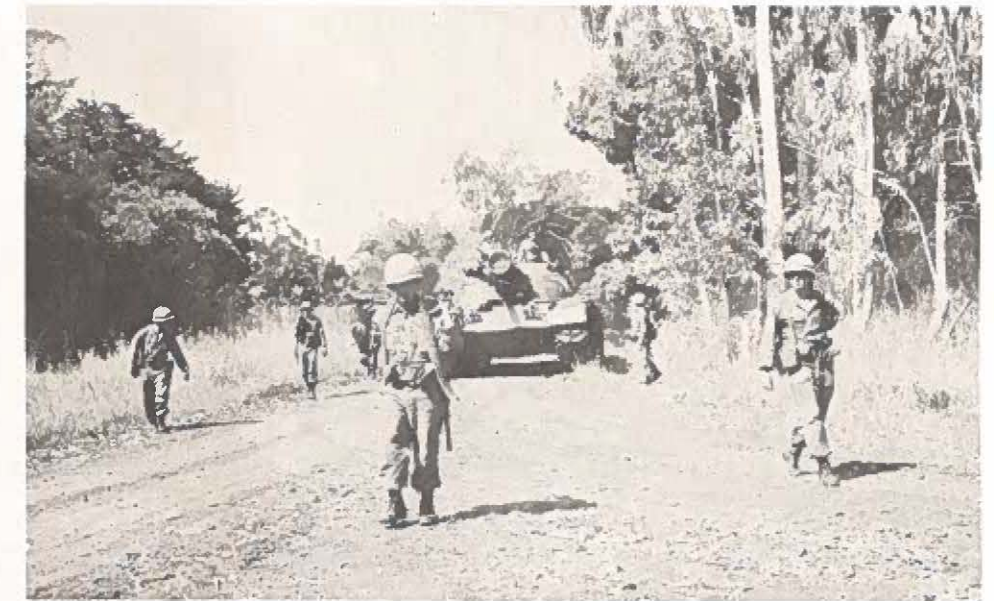
Tank support problems were interesting, tough. New tank, borrowed from 25th Infantry Division, has new type searchlight mounted above tank gun which operates in unison with gun.
