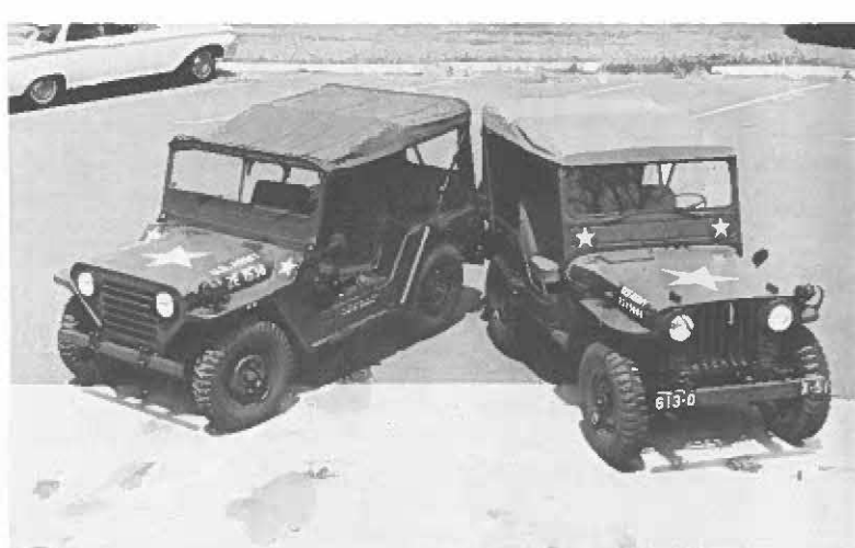
NEW JEEP (left) will gradually replace old model (right) within the HARNG. Nine of the 4X4 M-151 quarter-ton Willys' jeeps have been delivered to the Guard thus far. The four-cylinder vehicle (with overhead valves) costs $3,790.00 and has independent suspension.
