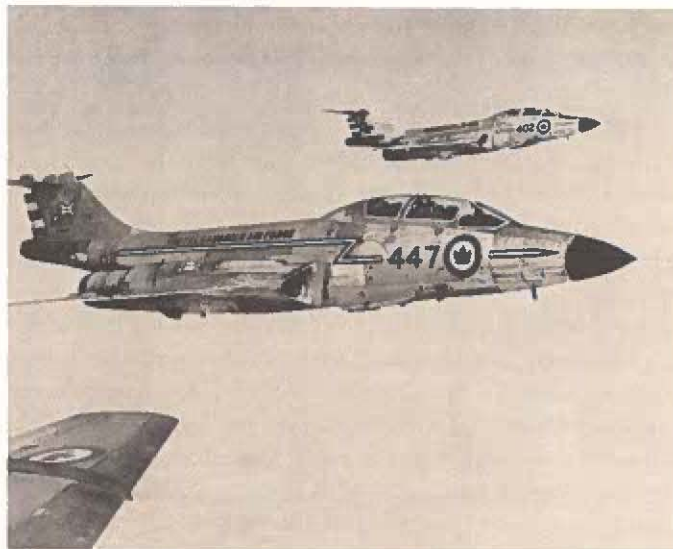
ROYAL CANADIAN Air Force flies supersonic CF-101B Voodoo. Long range fighter is armed with air-to-air Falcon missiles and Genie rockets.
