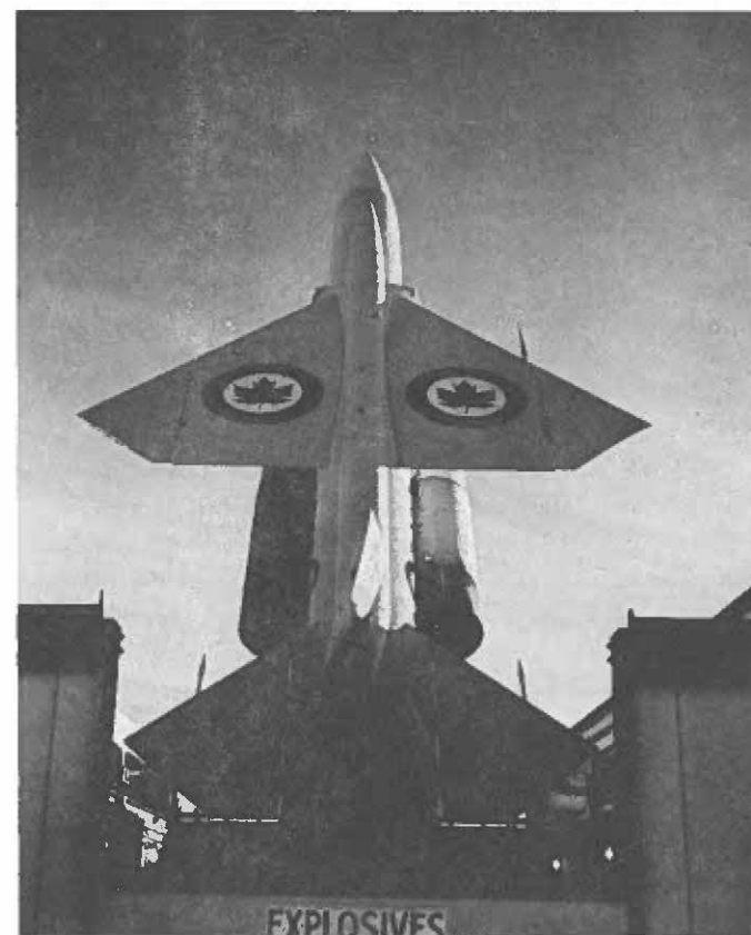
CANADIAN BOMARCS add to defense of North America's industrial and population centers. Canada has two squadrons; U. S. has eight. Nuclear capable Bomarc "B" has range of 400 miles, flies at three times the speed of sound and can "home" on targets at altitudes near 100,000 feet.
