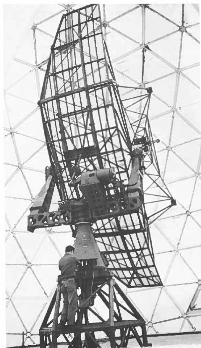
ONE OF TWO pieces of radar equipment in the giant, plastic domes atop Kaala is this height-finder. Plastic dome is 50 feet in diameter and can withstand winds in excess of 150 m.p.h.
