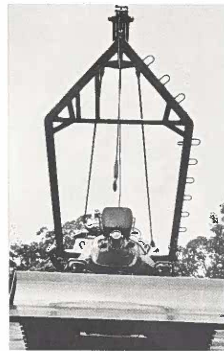
THE DESTRUCTOR — The engineers have a name for it, and it is officially known as the M728 Combat Engineer Vehicle (CEV). The weapon-tool is a combination bulldozer, crane and tracked artillery vehicle. Using the chassis and armor of the M-60 tank, the CEV's special 165mm cannon can hurl a shell filled with plastic explosive more than 1,000 meters. The big shell, which is completely self-contained with no outer casing, is used to demolish fortifications. Its 100 million candlepower searchlight makes it useful for night operations. The first of these to be deployed outside North America are now being used by the 227th Engineer Co, 29th Inf Bde. (U. S. Army photo)
