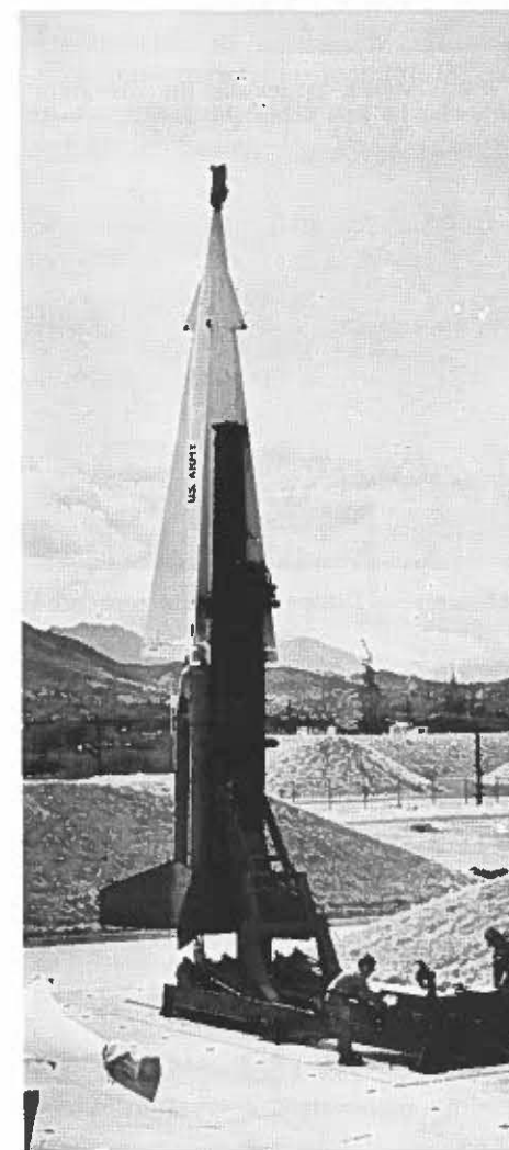
TWO MEMBERS OF BTRY C'S LAUNCHER PLATOON perform maintenance checks on a Nike-Hercules Missile and Launcher.
